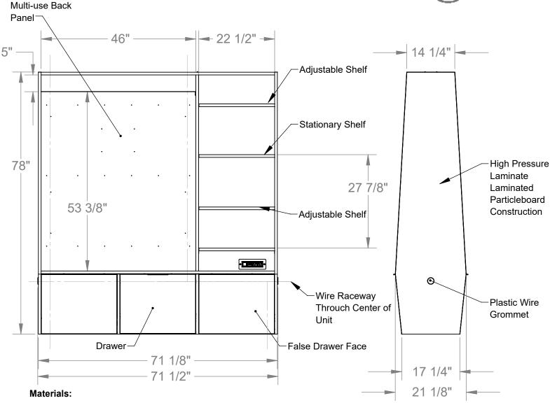
• Panels: 3/4" thick high pressure laminate laminated particle board.
