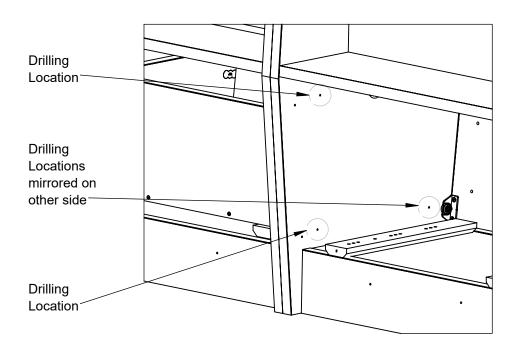
Step 4: Connect a 1/4"-20 x 1-1/2" bolt with a 1/4"-20 barrel nut at all four holes locations drilled in step 3. Tighten bolts together using a 5mm and #2 phillips bit.
